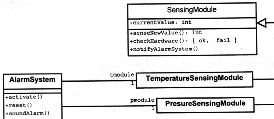
will do so *concurrently*. To start up, each will run a check on tis own hardware. This may take a while. If successfull then it goes over the 'ready' state. Only when both modules are in the 'ready' state, then the whole system is in de 'ready' state.
