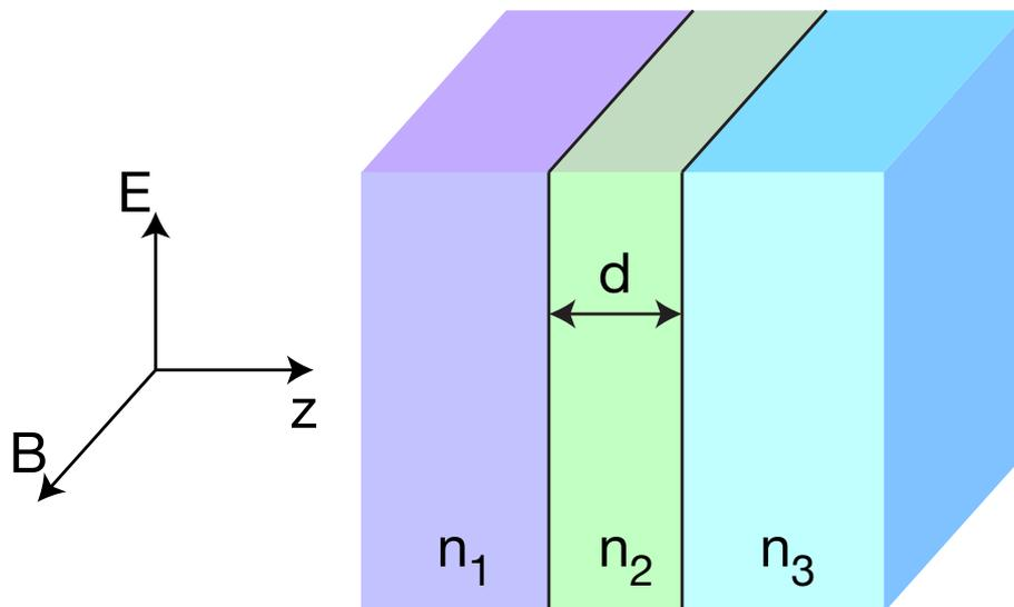
have  $\vec{E}_I = \vec{E}_0 e^{i\vec{k}_1 \cdot \vec{r} - i\omega t} + \vec{E}_1 e^{-i\vec{k}_1 \cdot \vec{r} - i\omega t}$ , in the intermediate region (with  $n_2$ ) we have  $\vec{E}_{II} = \vec{E}_2 e^{i\vec{k}_2 \cdot \vec{r} - i\omega t} + \vec{E}_2 e^{-i\vec{k}_2 \cdot \vec{r} - i\omega t}$  and on the right (with  $n_3$ ) we have the transmitted one given by  $\vec{E}_{III} = \vec{E}_3 e^{i\vec{k}_3 \cdot \vec{r} - i\omega t}$ .
