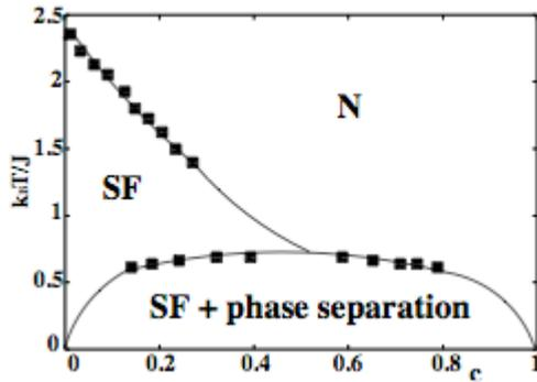
Figure 1: Phase diagram of the Blume-Energy-Griffiths model, obtained by Monte Carlo simulations.  $N$  denotes the normal phase,  $SF$  the superfluid phase.
