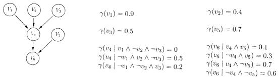
Variables  $V_1, V_2$  and  $V_3$  have a disjunctive interaction effect on variable  $V_4$ . To capture this effect, the assessment function for node  $V_4$  is based on the 'noisy-or gate'.
