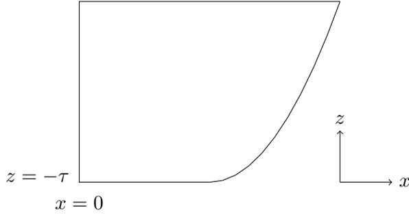
Critical points exist in the three acute corners (which have 'all' inclinations) and in one point on the parabolic bottom where its slope equals 1, namely at  $(x_c, z_c) = (\frac{1}{2}(1 + \frac{1}{4\tau}), -\tau(1 - \frac{1}{16\tau^2}))$ , provided  $x_c > 0$ , i.e. provided  $\tau > \frac{1}{4}$ . For smaller  $\tau$ -values the bottom is everywhere subcritical and the corner  $(1, 0)$  attracts. In that case there are only 3 critical points (the corners).
