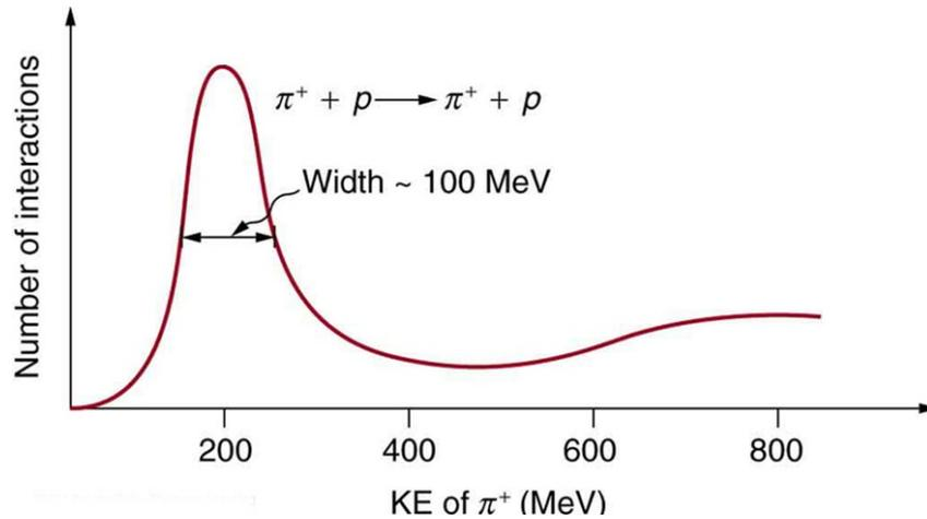
Figure 5: The probability of the interaction between a  $\pi^+$  and a proton as a function of the incident kinetic  $\pi^+$  energy.
