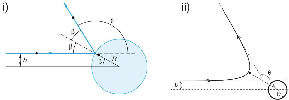
Figure 1: i) Diagram should show scattering at approximately correct angle and with angle of incidence approximately equal to angle of reflection.  $b$  and  $\theta$  must be indicated and defined as scattering parameter and scattering angle respectively.  $\beta$  and  $R$  are not required. ii) Path should have smooth curve resembling hyperbola at approximately correct angle.  $b$  and  $\theta$  must be marked.  $r_c$  and  $R$  are not required.
