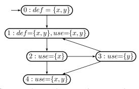
State 0 is the initial-state, and state 4 is the end-state. If no def or use is mentioned on a node, it means the corresponding decoration is empty on that node.
